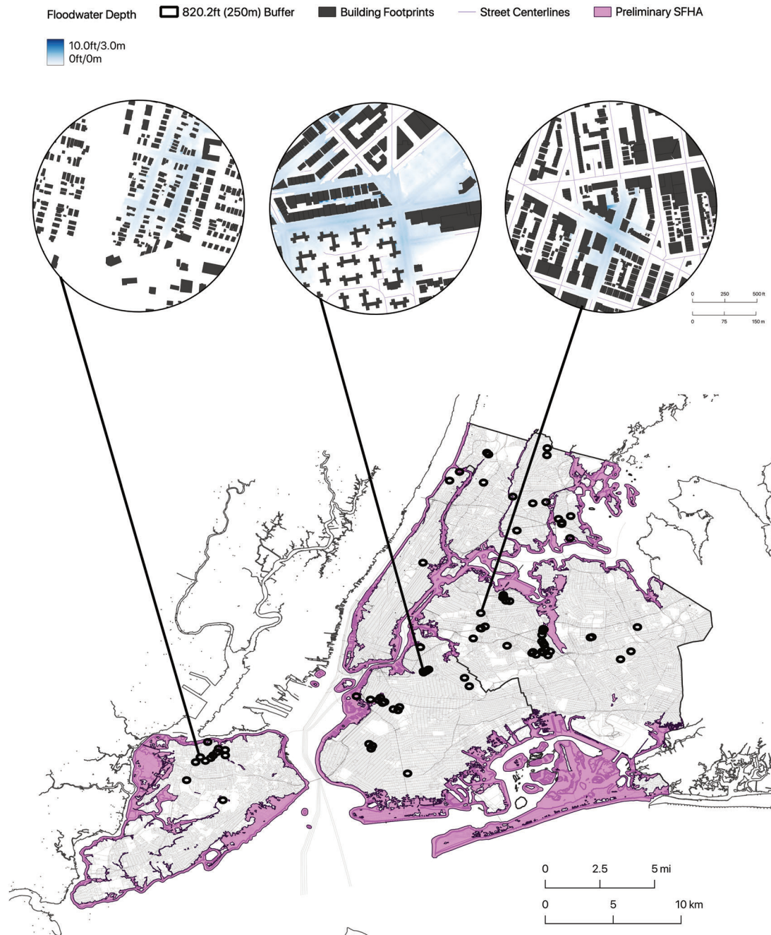
FIGURE 7 A total of 83 high water marks (HWMs), such as seed lines, mud, and debris, were surveyed by the US Geological Survey in the weeks following the Ida Remnants Cloudburst. 135,136 Using these observations, land surface inundation was estimated within an 820.2 ft (250 m) buffer of each observed HWM. During the Ida cloudburst, deep inundation from pluvial flooding occurred in areas that were far from the water bodies used as the basis of Federal Emergency Management Agency Special Flood Hazard Areas (FEMA SFHA) modeling. Flooding from this event was not limited to areas where HWMs were obtained and occurred in areas of the city that were not surveyed or where HWMs could not be identified. Several inundated areas are highlighted here, and all HWM data from this survey can be viewed at: https://stn.wim.usgs.gov/fev/#2021lda . Figure by: BR Rosenzweig.
